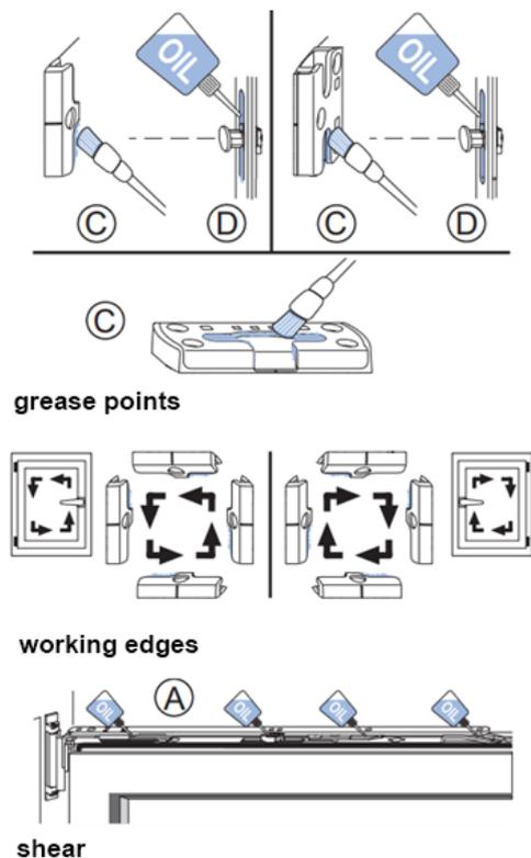
Figure 1 shows possible lubrication points that should be lubricated at least once per year.
